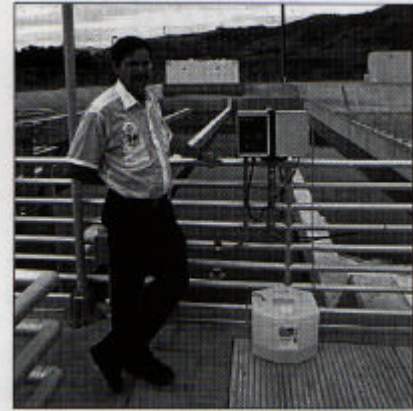
Each sensor is equipped with an optional self-cleaning kit which periodically rinses the probe in a mild solvent solution.
